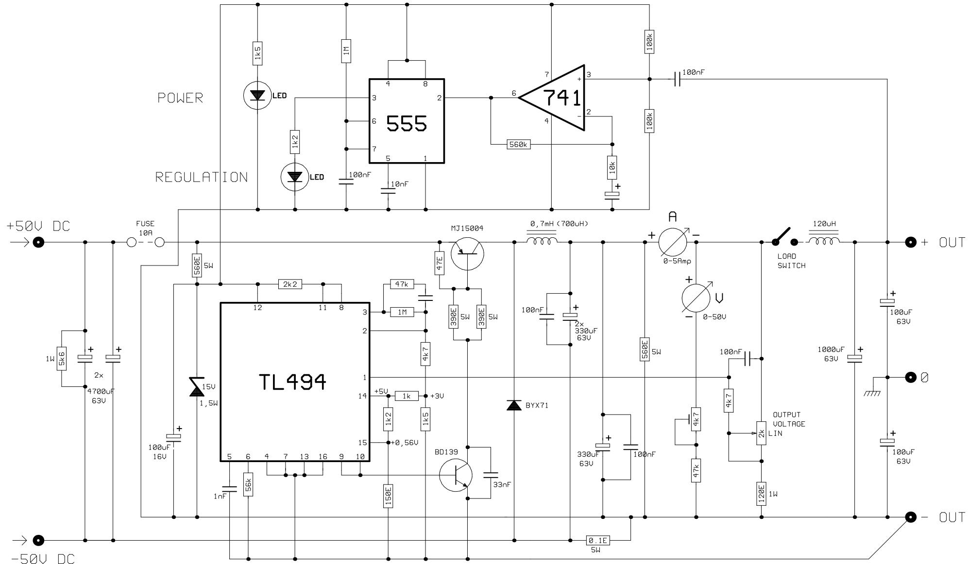
0-50V/5Amp Switch Mode LAB PSU
